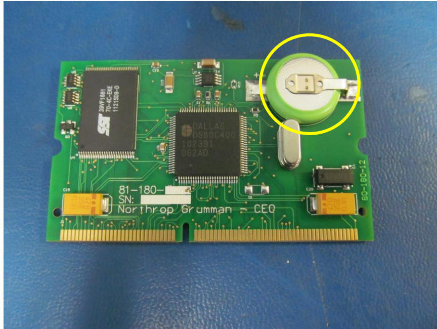
Figure 2: TINI Circuit Board Battery Location
